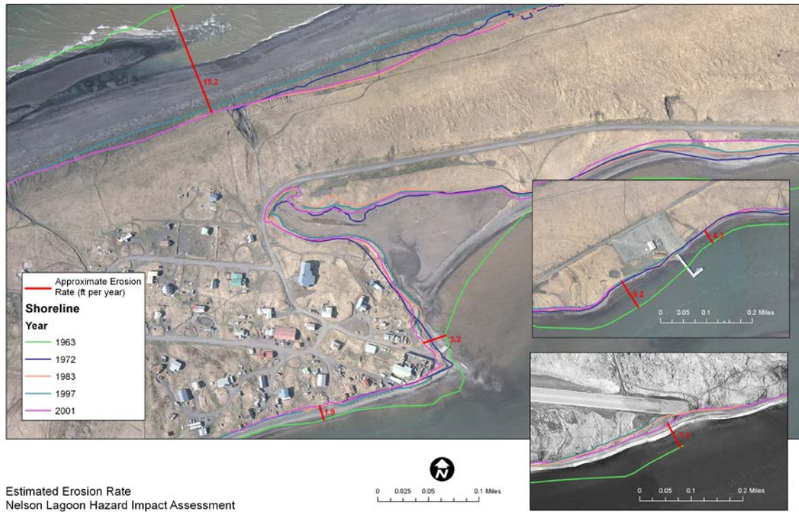
Figure 25. Approximate Erosion Rates
